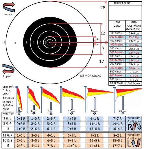
0.308 cal, 155 grain, HBC (R&J Sports goods), G1 BC 0.462, Muzzle velocity 2950 Fps, 13 to 1 Rh twist barrel, Station Pressure 1000 Hpa, 75% Humidity, 30 Degrees Celcius.
