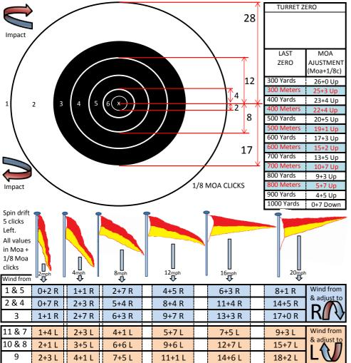
0.224 cal, 80 grain, Hornady A-Max, G1 BC 0.453, Muzzle velocity 2960 Fps, 1 in 8" Rh twist barrel, Station Pressure 1000 Hpa, 75% Humidity, 30 Degrees Celcius.
